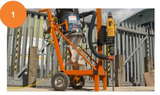
Sindrilla is weighted, not mechanically driven. Its smart design means there are no complicated technical components involved making Sindrilla easy to maintain.
